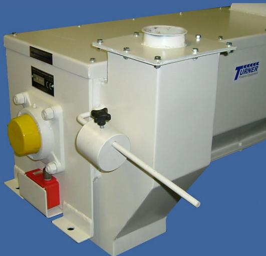
Fabricated in mild steel, the outer housing encloses a horizontal main shaft onto which is fitted a series of beater bars. The unique distributed pattern of the beater bars ensures correct product flow through the unit whilst maintaining both productivity and efficiency.
