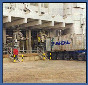
The Turner Bulk Container Loader has for many years been utilised for the loading of malt and fish meal products into lined bulk containers. As with many bulk materials malt products require a system that can handle product in a gentle manner whilst providing efficient loading characteristics to maximise the useful volume available within a lined container.
