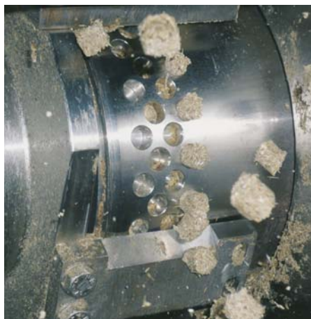
Pressure and temperature build-up with the KAHL expander technology
